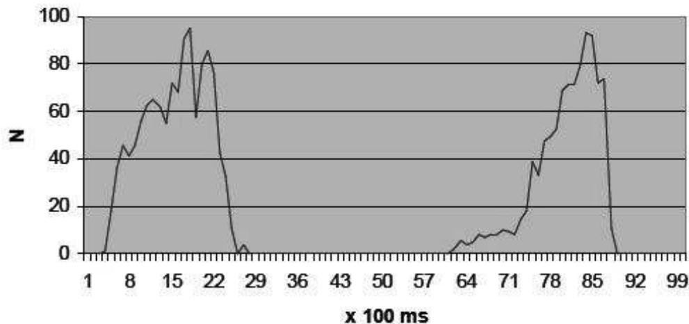
Fig. 4. Thrust force of drilling of cortical bone.
