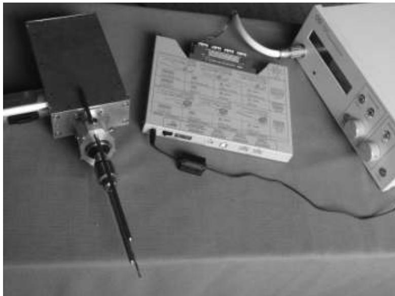
Fig. 1. A bone drilling experimental set up.
